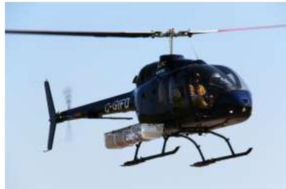
Designed for both utility and VIP operations, the Bell 505 Heli-Utility-Basket™ offers quick and easy installation and provides a safe, external solution for carrying skis, cargo hooks, tools, equipment, and a wide range of mission-essential items. The basket is constructed from corrosion-resistant stainless steel and finished with a high-gloss, scratch-resistant white coating for long-term durability and a clean appearance.
