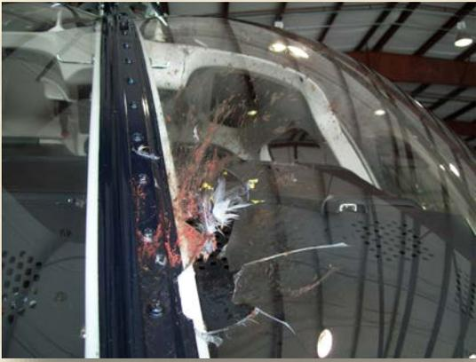
**Cockpit glass** upgrades are another interesting approach to reducing the severity of hitting a bird in flight. One state police aviation unit had six bird strikes in two years, two of which penetrated into the cockpit. The agency decided to mitigate the risk involved in future incidents by installing polycarbonate canopies in their Bell 407s.
