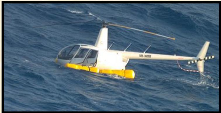
Without the recovery of the helicopter, the reasons for the partial engine power loss could not be conclusively determined. However, the indications were consistent with a magneto/governor failure, on which Robinson Helicopter Company has published a revised service letter *Governor troubleshooting / magneto maintenance* describing how the failure occurs and the compliance procedure.
