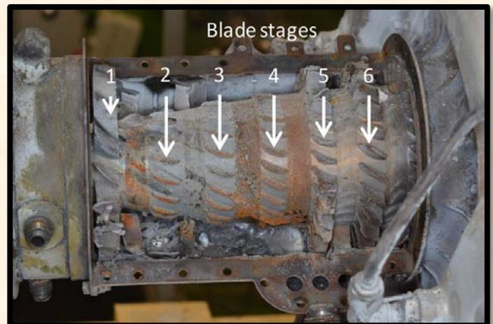
to the front support struts or to the stage 1 compressor blades suggests that the engine did not ingest any foreign objects.
