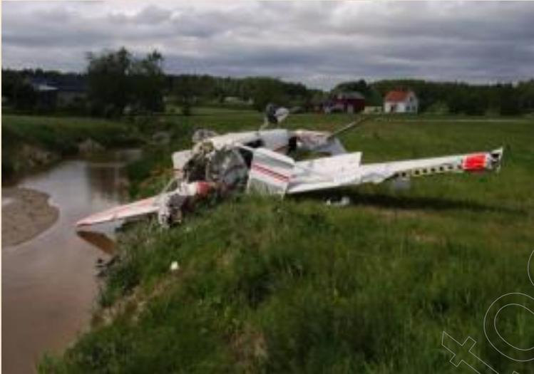
In connection with lowering the flaps and climbing, however, the speed reduced so far as to come below stalling speed, whereupon the aircraft dropped its left wing and entered a spin. During this turn the aircraft was influenced by an increasing tailwind, which exacerbated the situation.
