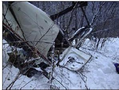
Aircraft impacted inverted and seatbelt failed... No head injuries to the survivor.
