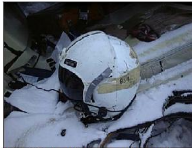
Aircraft impacted inverted and seatbelt failed... No head injuries to the survivor.
