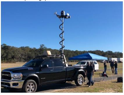
DroneSentry-C2<sup>TM</sup> ingested the data from several sensors. including the radar, radio frequency (RF), and our TrakkaCam TC-300 to provide an intuitive visualization of and potential airspace drone threats.
