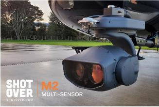
firsts to airborne ISR, the M2 Multi-Sensor system comes with SHOTOVER's 5<sup>th</sup> generation, true 6-axis gimbal design and is the only EO/IR system that eliminates "gimbal-lock" and "horizon-rolling".
