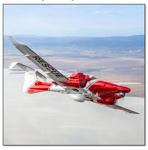
The TrakkaCam TC-375's EO/IR sensors are augmented with sophisticated image processing to see through environmental conditions like fog, haze, low light, and total darkness. A high-speed, digital video engine embedded is directly within the single-LRU gimbal delivering several standard optional functions; Moving Target Indicator (MTI) with Drone Detection Mode, which increases system performance and reduces operator workload.
