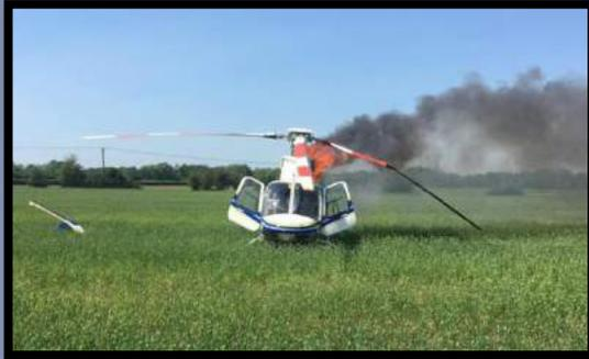
The pilot estimated that approximately 27 seconds had elapsed after the second caution light when there was a “mechanical snapping noise”, a violent yaw to the left, the red engine out warning illuminated, the torque dropped to 3% and a horn was heard. He realized the engine had failed and immediately “fully” lowered the collective and moved the cyclic control rearwards to slow to 60 kt.
